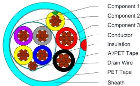
Component 2 Component 3 Conductor Insulation AI/PET Tape Drain Wire PET Tape
